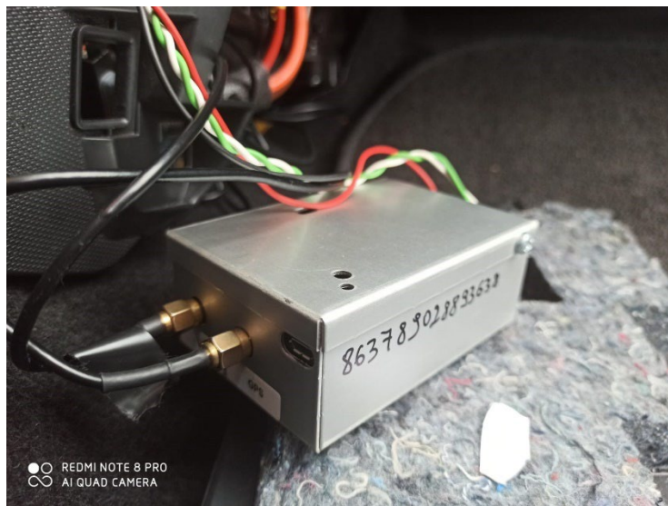
Figure 80: On-Board Diagnostic Device (OBD) connected to EV diagnostic interface
