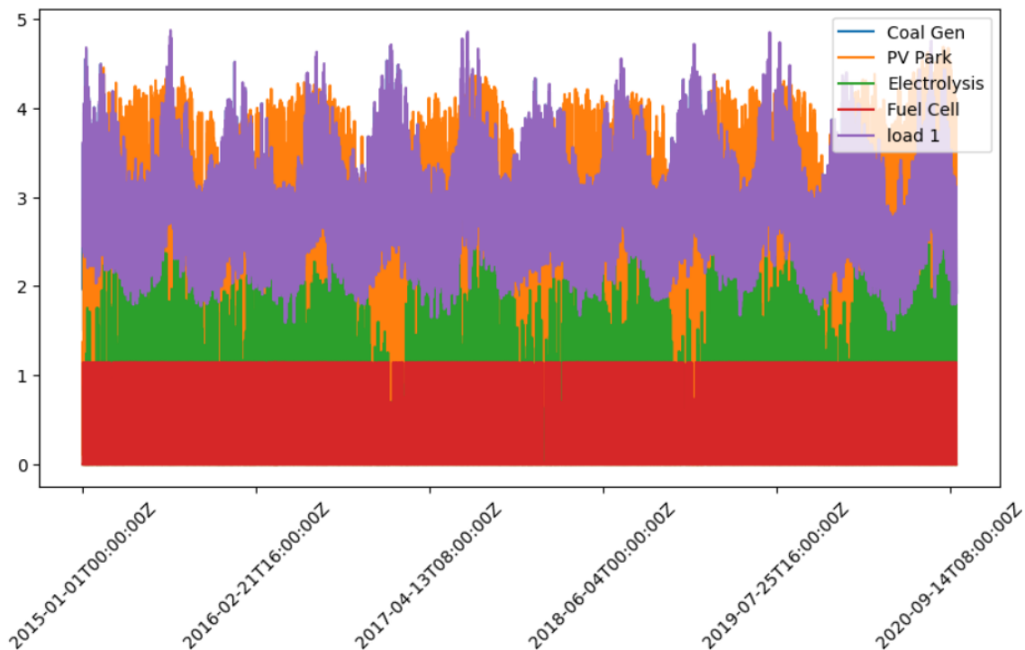
Figure 66: Load, generation, electrolysis, and fuel cell active power (MW) within the power system of scenario 2 for the simulation horizon (20150101-20200930)
